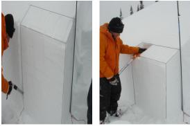
Fig. 2: Isolating an ECT column (left) and loading the column in the same manner as the compression test (right).
