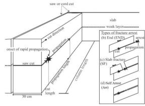
Fig. 1: PST column schematic with observable result types.
